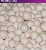
granule 2,5 - 5,0 mm Shape Bulk density 0,64 kg/l
