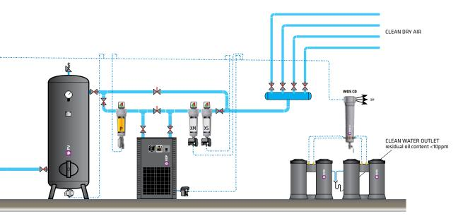
Drain valves are installed on moisture separators, coalescing filters, air receivers, air dryers and drip legs to remove this condensate from the compressed air system. The condensate should be piped from automatic drain valves to oil/water separators to remove the oil from the condensate before it is discharged into a drain. Make sure, that the drains operate properly. This is the only way to ensure that the filters and separators are successful in completing their task.
