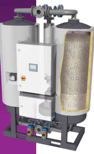
Adsorption compressed air dryers are a type of compressed air dryer that uses an adsorbent material to remove moisture from compressed air. Unlike refrigeration compressed air dryers that use cooling to remove moisture, adsorption dryers use a desiccant material to adsorb moisture from the compressed air.
