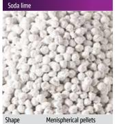
Menispherical pellets Bulk density 0,93 kg/l
